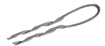
The OFT-PGG7 XXX preforms are made up of 7 powerful helical ASTM A36 steel wires to evenly distribute the gripping force and tension, their anti-corrosion process is based on the ASTM 123 hot-dip galvanized standard. The OFT-PGG7 XXX is designed for the perfect anchoring of ADSS cables in the deployment of FTTX networks.
