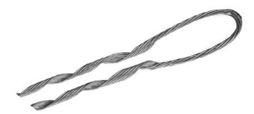
The OFT-PGG6 XXX preforms are made up of 6 powerful helical ASTM A36 steel wires to evenly distribute the gripping force and tension, their anti-corrosion process is based on the ASTM 123 hot-dip galvanized standard. The OFT-PGG6 XXX is designed for the perfect anchoring of ADSS cables in the deployment of FTTX networks.
