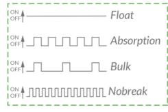
**Stages of the battery charger:** Indicated on the front panel, are symbolized by a LED that turns on and off according to the behavior shown in the figure on the right.
