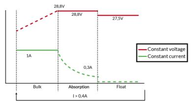
The graphic above shows the charging stages of the battery charger, illustrating the voltage and current behavior of the batteries as well as the migration point from one stage to the next. Current values might vary depending on the DC UPS model. Note: Graphic for the 24V/7A model
